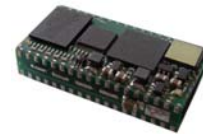
Type K3870: Centralized In-dummy DAQ system with non volatile flash data memory for maximum data security With Lion battery
